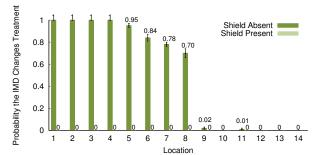
Figure 12—Without the shield, an adversary using an off-the-shelf programmer to send unauthorized commands (in this case, to modify therapy parameters) succeeds with high probability. The shield materially decreases the adversary's ability to control the IMD.
