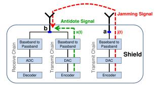
Figure 2—The jammer-cum-receiver design uses two antennas: a jamming antenna that transmits the jamming signal, and a receive antenna. The receive antenna is connected to both a transmit and receive chain. The antidote signal is transmitted from the transmit chain to cancel out the jamming signal in the receive chain.
