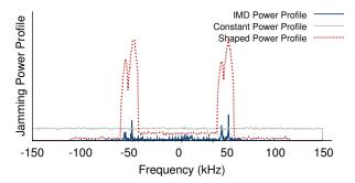
Figure 5—Shaping the jamming signal's profile to match an IMD's allows the shield to focus its jamming power on the frequencies that matter for decoding, as opposed to jamming across the entire 300 KHz channel.
