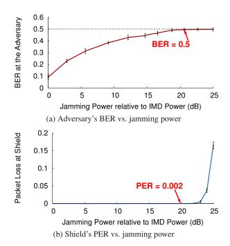
**Figure 8—Tradeoff between BER at the eavesdropper and reliable decoding at the shield:** If the shield sets its jamming power 20 dB higher than the power it receives from the IMD, it can ensure that an eavesdropper sees a BER around 50% (a)—effectively reducing the eavesdropper to guessing—while keeping the packet loss rate (PER) at the shield as low as 0.2% (b).
