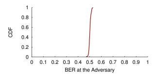
Figure 9—CDF of an eavesdropper's BER over all eavesdropper locations in Fig. 6: At all locations, the eavesdropper's BER is nearly 50%, which makes its decoding task no more successful than random guessing. The low variance in the CDF shows that an eavesdropper's BER is independent of its location.
