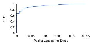
**Figure 10—Packet loss at the shield:** When the shield is jamming, it experiences an average packet loss rate of only 0.2% when receiving the IMD's packets. We conclude that the shield can reliably decode the IMD's transmissions despite jamming.
