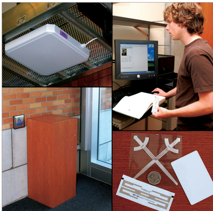
Figure 1. The RFID Ecosystem. RFID reader antennas are mounted on cable trays (upper left) and in custom-built wooden boxes (lower left). An RFID kiosk (upper right) lets users associate one of three types of tags (lower right) with a personal object.
