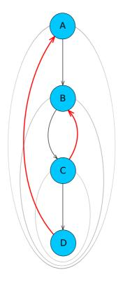
Figure 2.8: If the conflicting edge C—B is resolved before D—A, then the edges B—C and C—B will have to be revisited.
