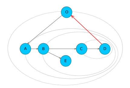
Figure 2.6: Objects O, A, B, C and D will be made peer. Object E stays in the context of B.
