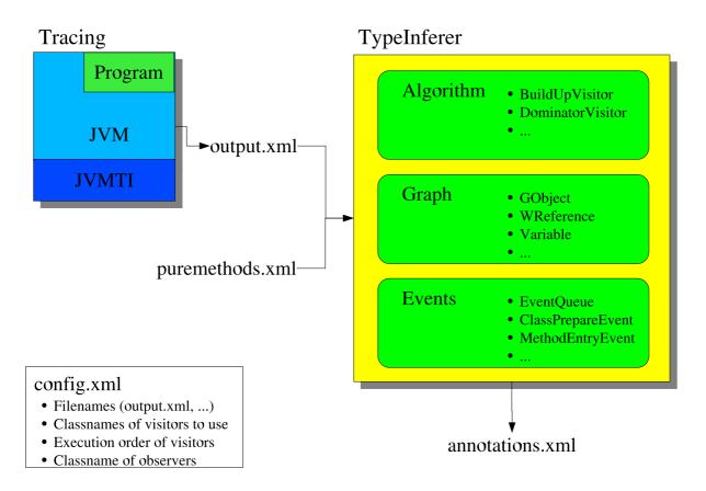
Figure 3.1: The overall architecture.
