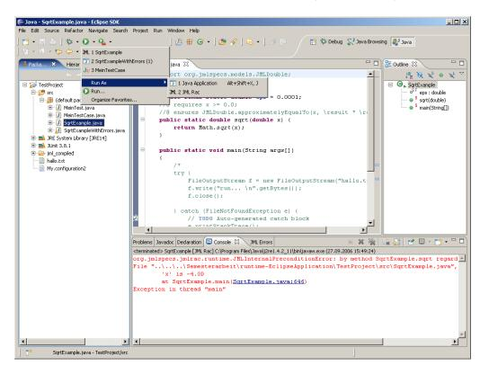
Figure 3.2: Run JML runtime assertion checker
