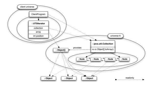
Figure 5.6: An example runtime object structure with a UTSIterator.
