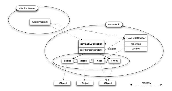
Figure 3.2: Collection and according iterator, like provided by the Java API.
