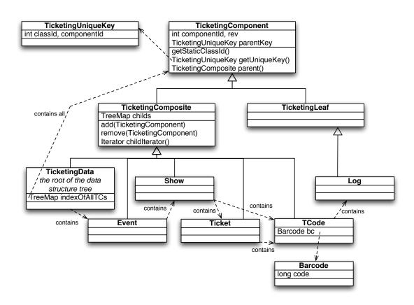
Figure 1.4: Class diagram of the data structure classes. These classes implement the composite pattern.
