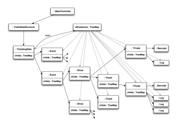
Figure 1.3: An example runtime object structure of the Data Structure component. allInstances is a static field in the class TicketingData and represents the index over all components in the tree; references of this index are drawn with grey arrows.
