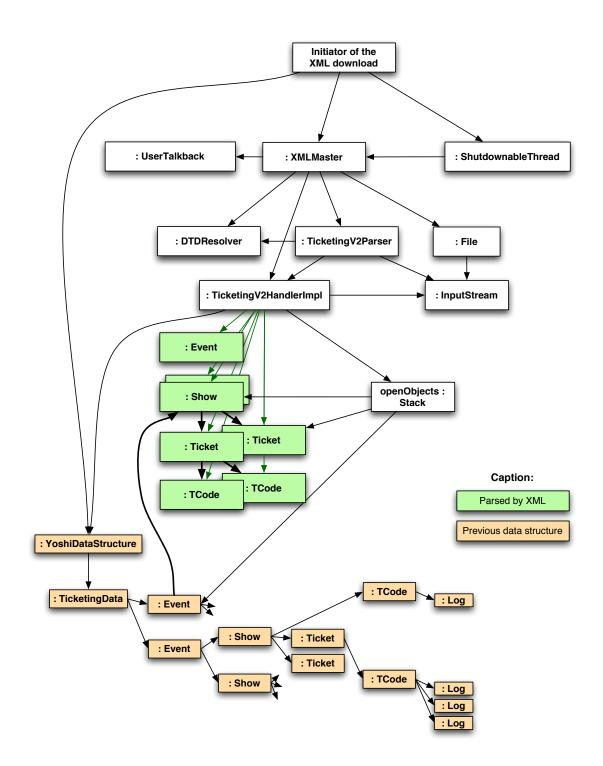
Figure 4.6: An example runtime structure of the XML Download before any universe annotations. It shows the object structure of a download of an XML, where a show is added to an existing event. Bold arrows mark references added to the Data Structure by parsing the XML.
