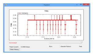
Figure 6: Real-time Plotting Utility Reporting Current Consumption.
