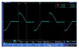
Figure 12: Plot of voltage across the terminals of the CFL with dimmer level set to 50.
