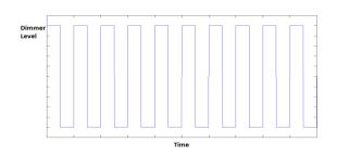
Figure 9: Periodic rectangular pulses applied to CFL. Plot of Z-Wave dimmer level versus time.
