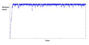
Figure 10: Random Gaussian distributed signal applied to CFL. Plot of Z-Wave dimmer level versus time.
