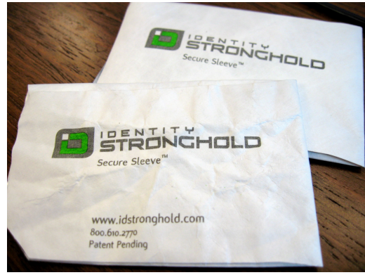
Figure 3: The sleeves used for our shielded distance tests. The crumpled sleeve is in the foreground, with the new sleeve behind it.
