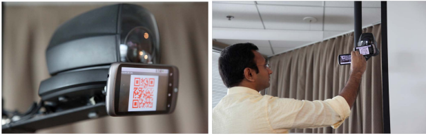
Figure 1: The QR Code encodes the camera’s recent activity and data retention policy (left). An individual reviews the privacy report using a barcode reader mobile application (right).
