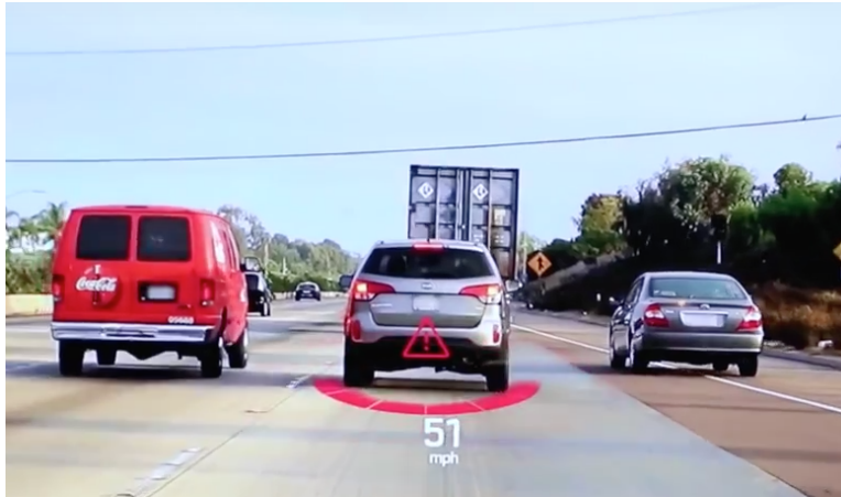
Figure 3.1: Example AR Scenario. This screenshot from Hyundai’s CES demo [53] shows an AR warning overlaid on a car and the car’s current speed.
