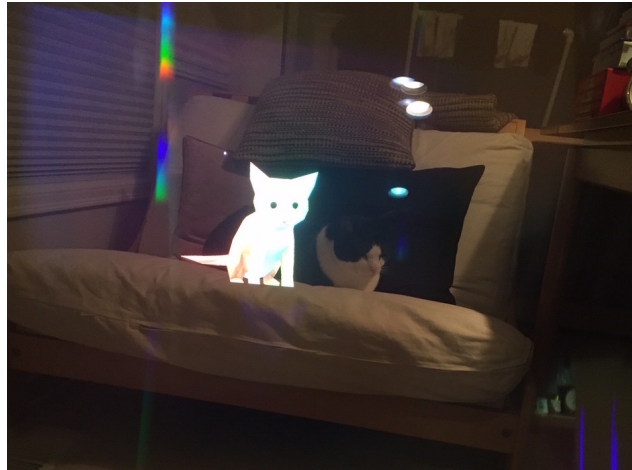
Figure 3.2: Real-World Occlusion. This photo was taken by a smartphone through a HoloLens display (resulting in some reflective camera artifacts). It shows that virtual content displayed by HoloLens (here, a cat) can visually obscure real-world objects (also a cat).
