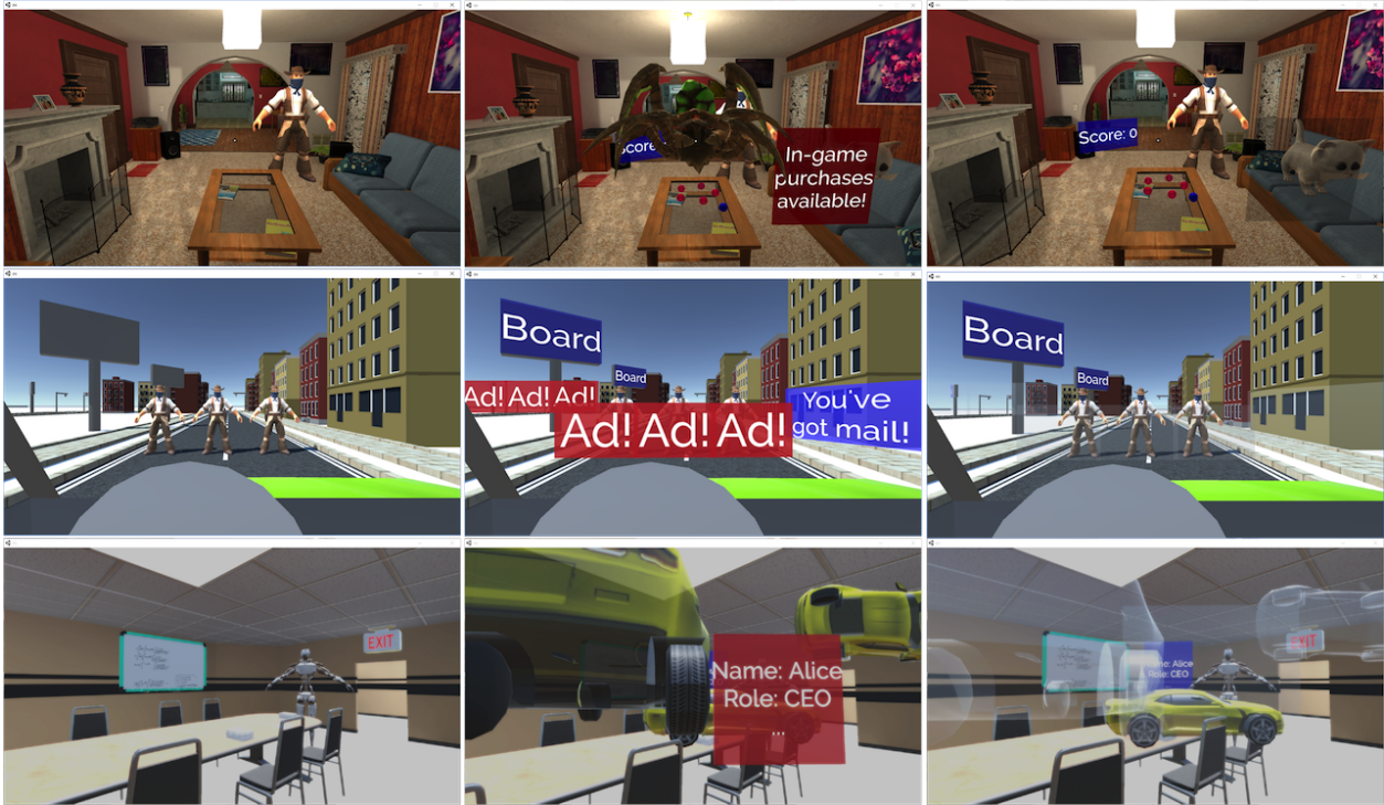
Figure 3.6: Case Studies. These screenshots show our case study scenarios: HMD in the home (top), car windshield (center), and HMD in the office (bottom). The left column shows the bare scenes in our Unity-based AR simulator, representing the real world without any apps running. From our prototype’s perspective, everything in the bare scene is part of the real world. The center column shows our case study apps running, exhibiting both desirable and undesirable AR output behaviors. The right column shows the result of policy enforcement, leaving only desirable AR output. Note that Unity’s alpha adjustment mechanism leaves transparency artifacts to outline where violating AR objects would be.
