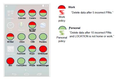
Figure 3.1. Examples of profiles with desired security policies
