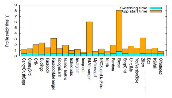
Figure 3.7. Time to switch an app between profiles
