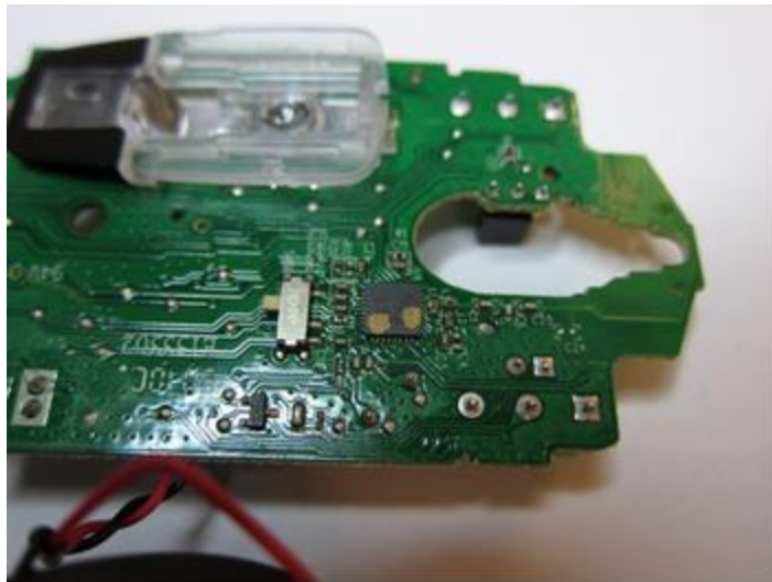
Figure A-2: Nordic nRF24L01 RF transceiver that is used on the Logitech mouse.
