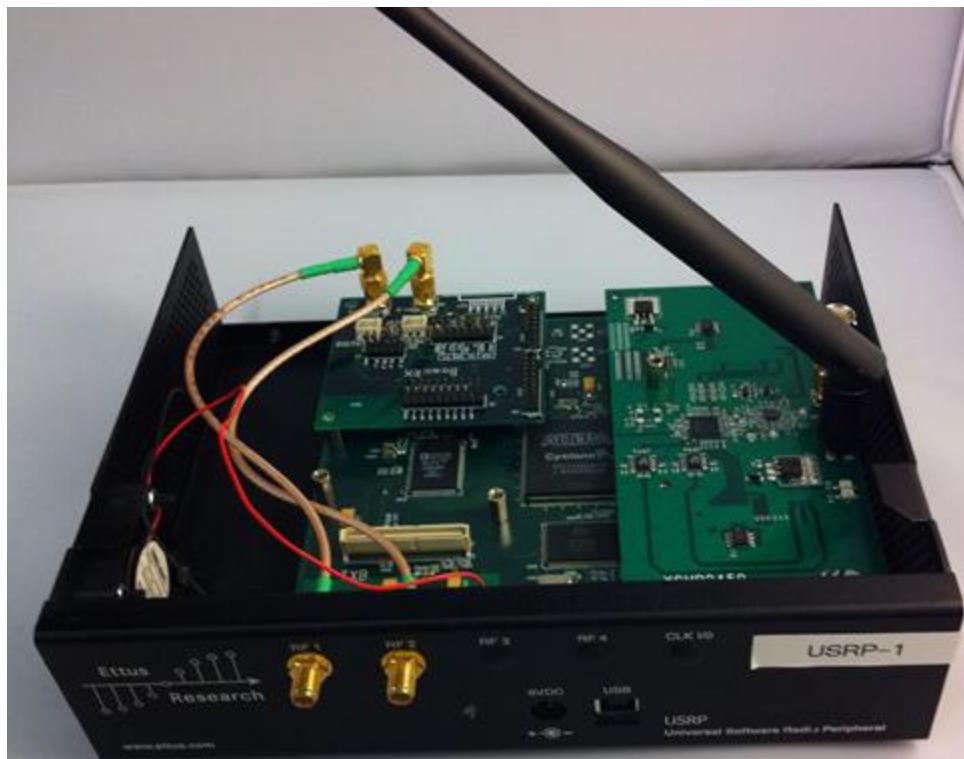
Figure A-4: USRP, a software radio platform that was used along with GNURadio for capturing RF signals.
