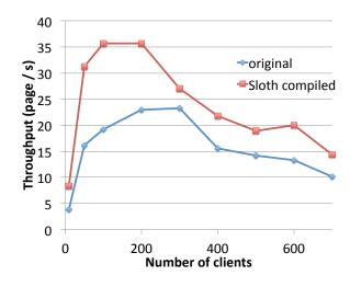
Figure 4-11: Throughput experiment results
