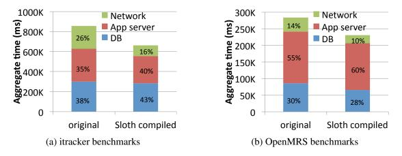
Figure 4-12: Time breakdown of benchmark loading experiments
