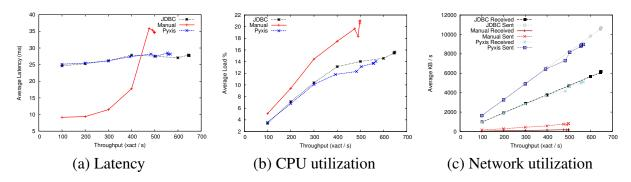
Figure 3-10: TPC-C experiment results on 3-core database server
