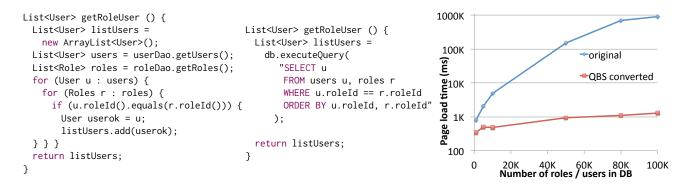
Figure 1-3: QBS results highlights: original code fragment (left); converted code fragment (middle); resulting performance comparison (right).
