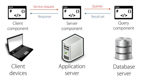
Figure 1-1: Software architecture of three-tier database applications
