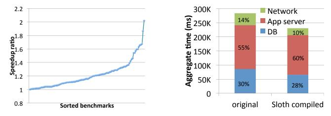
Figure 1-5: SLOTH results highlights: average page load speed up across 112 benchmarks (left); comparison of time breakdown in loading all benchmarks (right).
