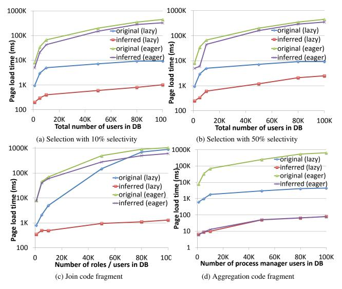
Figure 2-17: Webpage load times comparison of representative code fragments
