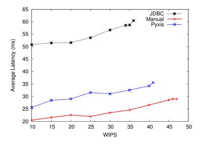
Figure 3-12: TPC-W latency experiment using 16 cores
