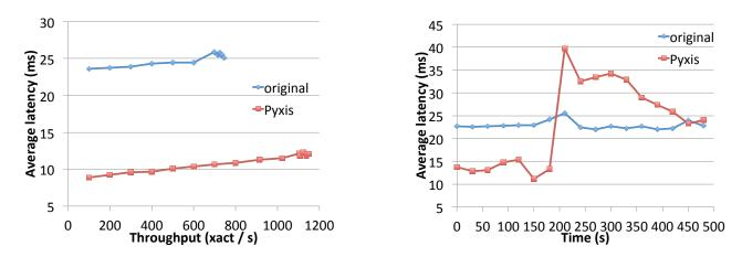
Figure 1-4: PYXIS results highlights: application latency with different throughput (left); application latency as the number of CPUs available decreased around 180ms (right).
