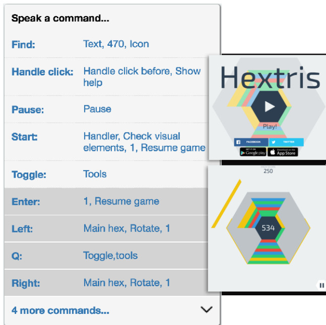
Figure 1. The Hextris web game (hextris.io) shown with a list of speech commands created by Genie. Speaking the bolded text label for each command triggers the corresponding actions.
