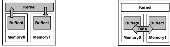
(a) Data movement controlled by kernel. (b) Data movement controlled by DMA.
