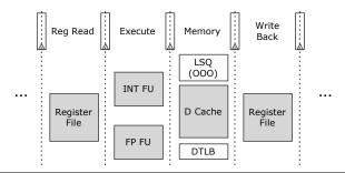
**Figure 1.** The data movement/processing plane of the processor pipeline. Approximation-aware structures are shaded. The instruction control plane stages (Fetch and Decode, as well as Rename, Issue, Schedule, and Commit in the OOO pipeline) are not shown.
