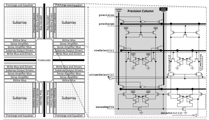
**Figure 2.** Dual-voltage mat, consisting of four identical dual-voltage subarrays, and partial transistor-level design of the subarrays and the *precision column*, which is shaded. The power lines during a read access are shown in bold.
