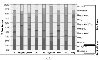
**Figure 6.** Percent energy consumed by different microarchitectural components in the (a) OOO and (b) in-order Truffle.
