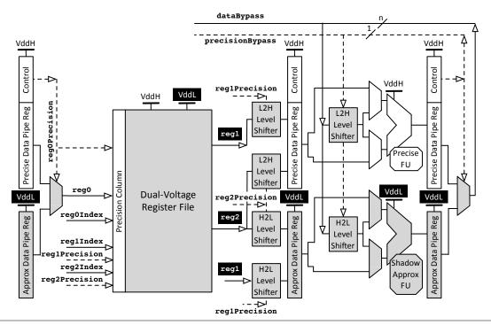
**Figure 4.** The register and execution stages in the Truffle pipeline along with the bypass network. The DV-Muxes and other approximation-aware units are shaded. The single-bit precision signals in the bypass network and in each stage are dashed lines.
