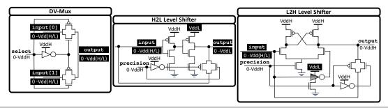
Figure 3. Transistor-level design of dual-voltage multiplexer (DV-Mux) and high-to-low (H2L) and low-to-high (L2H) level shifters.
