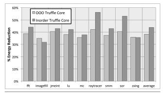
Figure 8. Percent energy reduction *potential* for checked in-order and OOO Truffle designs with  $V_{dd}L=0.75~\rm{V}$ .
