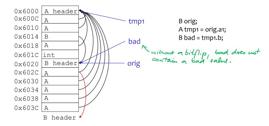
The heap has one A object, many B objects. All fields of type A point to the only A object that we need here. Place this object close to the many B objects.
