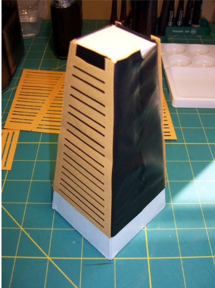
10. Attach the fourth rib section. It should be the same design as the one on the opposite side.
