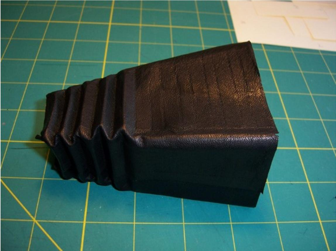
19. At this point I place the bellows face down on my work table and begin folding from the back. It is easier for me to do it this way since I can see how the folds need to occur and also allows me to use both hands to fold and push down on the table.
