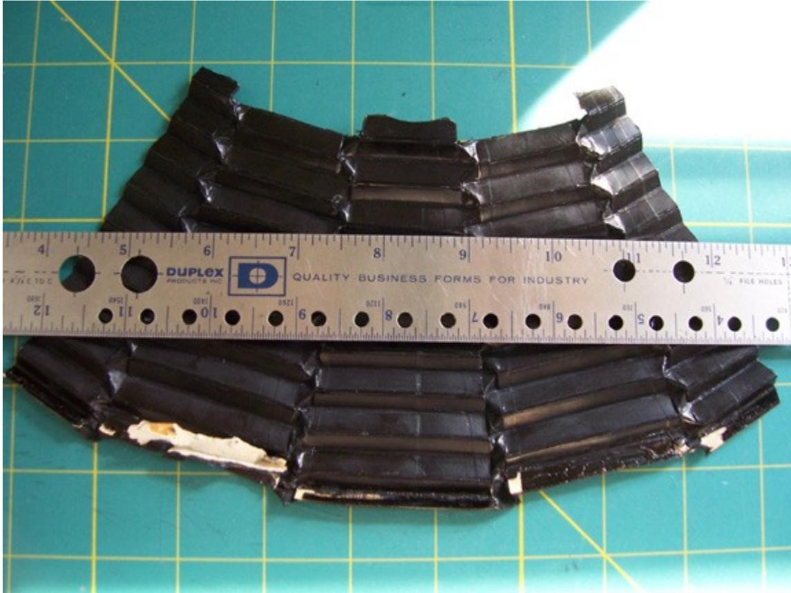
I usually trim the front of the bellows before inserting the brass front plate, but it can be done just as easily afterwards. I trim the back after mounting the bellows in the camera.
