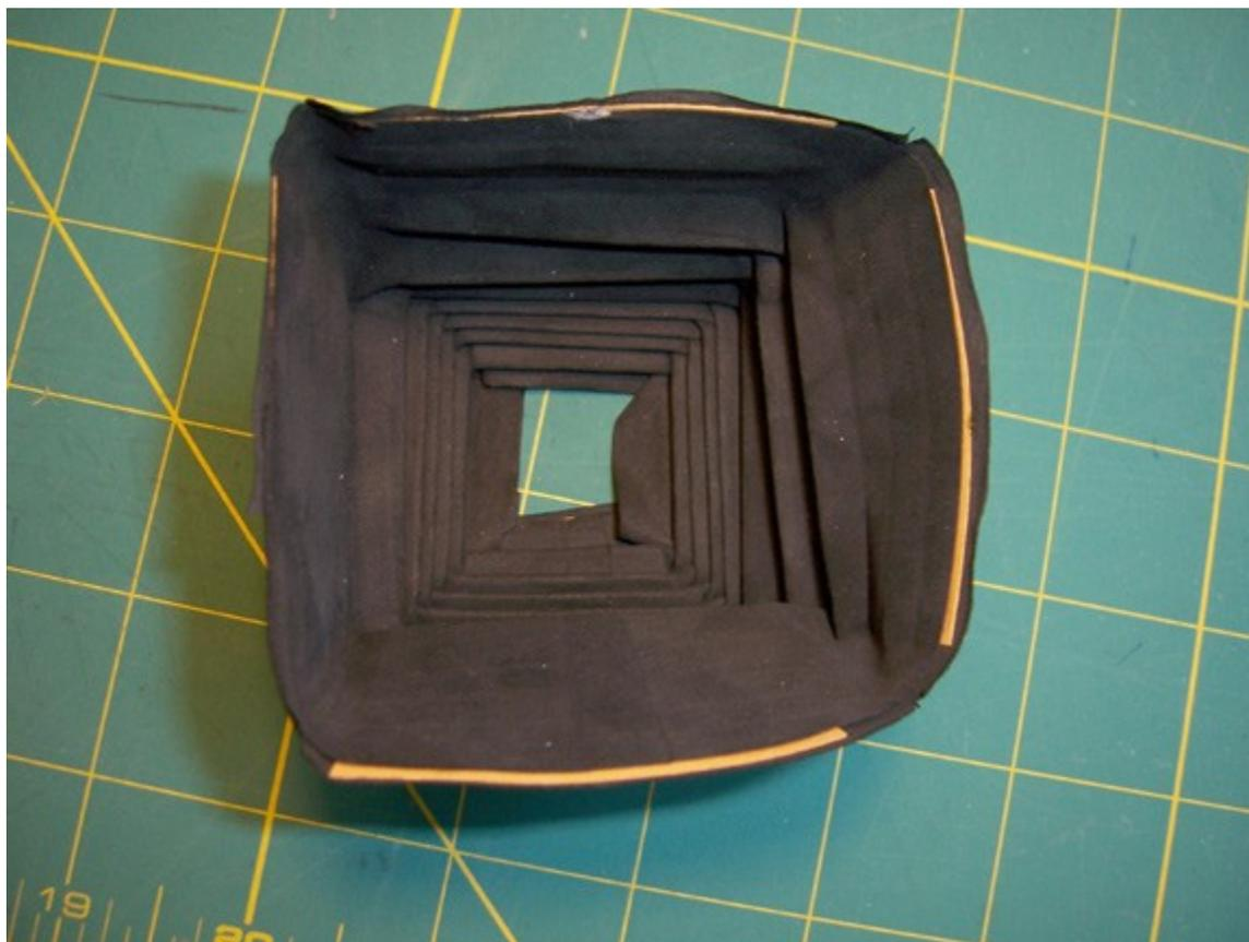
20. Here is the folded bellows (view from the back). After they are at this stage I recheck the folds and the corners and make any minor adjustments, then place a weight (not too much but just enough to hold them closed) on the folded bellows to set the folds.
