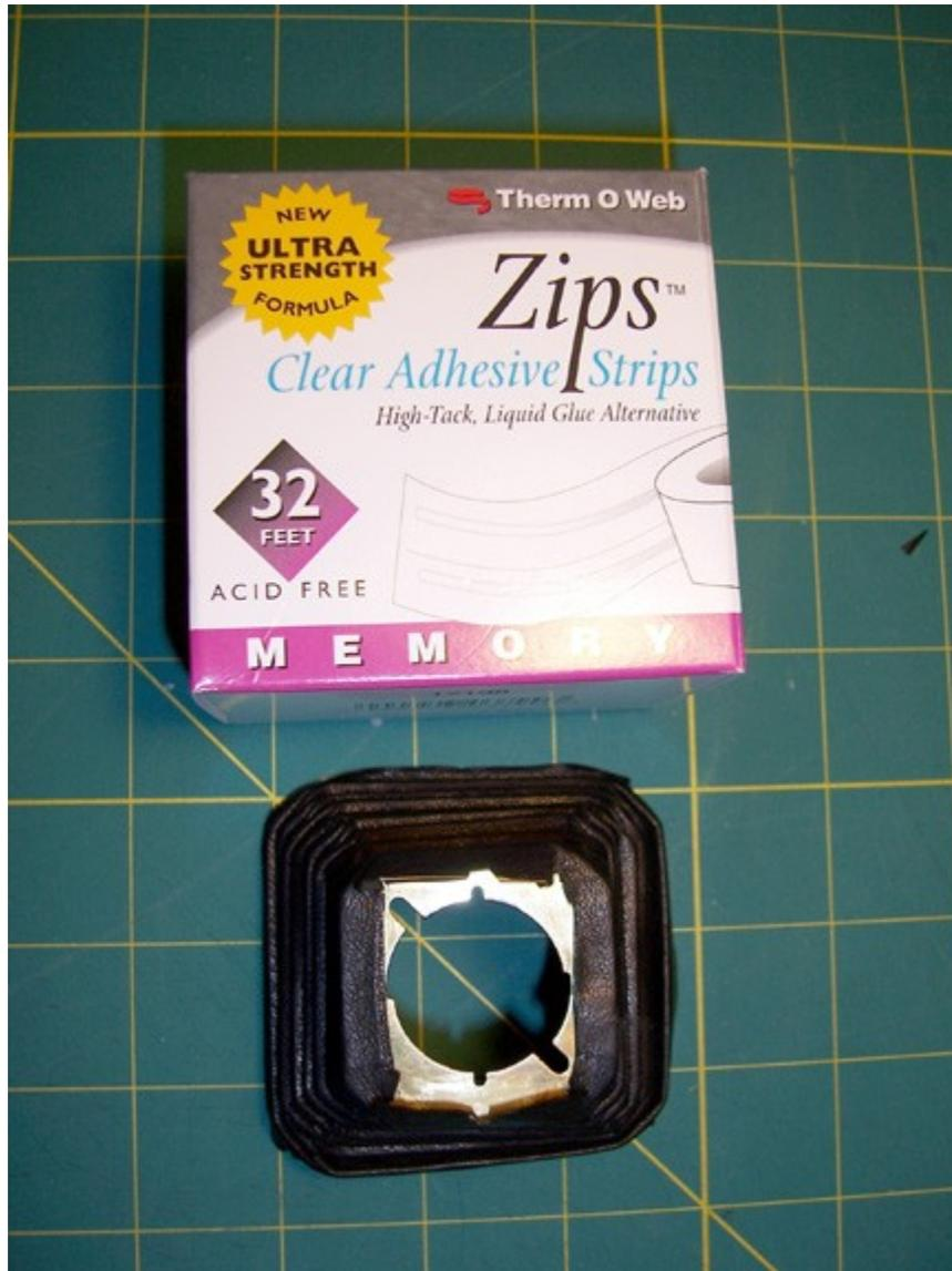
25. Here are the bellows read to mount. I still haven't perfected the overlapping corners as you can see. I sometimes have to do a little more trimming of the corners after gluing to the plate so that I have a relatively flat result to attach to the shutter.
