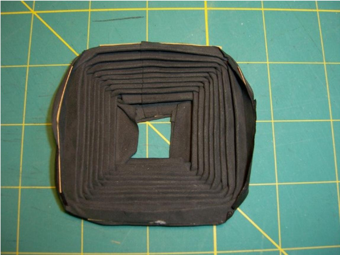
21. The next step is to mount the brass front plate, but first we need to look at the trimming of the bellows for mounting. Even though our bellows was constructed with equal length sides, as you can see in the following picture of a bellows removed from a camera, the first fold of the front portion of two of the sides has been removed. This is because the mounting of the bellows on the front plate (and also on the back portion at the film plane) has to result in adjacent folds being opposite.
