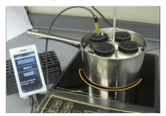
Figure 3: ODK Sensors deployment at a human milk bank in Durban. The application guides users through the pasteurization process by providing feedback based on temperature of breast milk (contained in jars that are heated).
