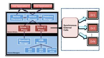
Figure 1: Architectural overview of ODK Sensors where a black rectangle represents a separate Android app. Top-level user applications leverage the framework's unified API to access sensor data. The framework communicates with sensor driver apps using Binder IPC (an Android service).
