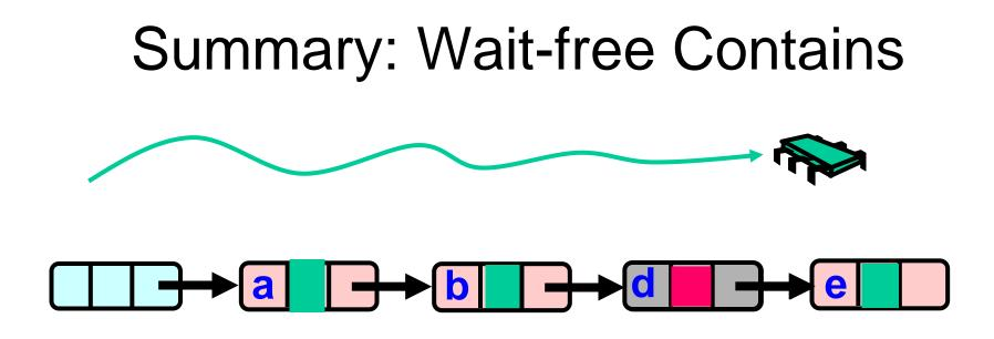
Use Mark bit + list ordering 1. Not marked  $\rightarrow$  in the set 2. Marked or missing  $\rightarrow$  not in the set
