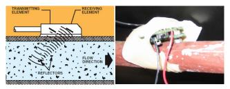
Figure 3. (left) A diagram of how ultra-sonic water meters work. (right) The audio-based water sensing system developed by Fogarty et al. (2006).
