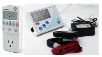
Figure 1. (left) The Kill-A-Watt plug-in load meter. (right) The Energy Detective uses sensors that clip-on to the home's main circuit breaker.
