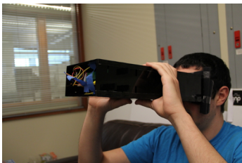
Figure 2: Viewing box prototype, inspired by approaches like Google Cardboard and modeled after the form of the Lafayette system. Slits on the side of the box to allow for variable distance between the light source and the person. The box can be rested on a surface while taking a test.
