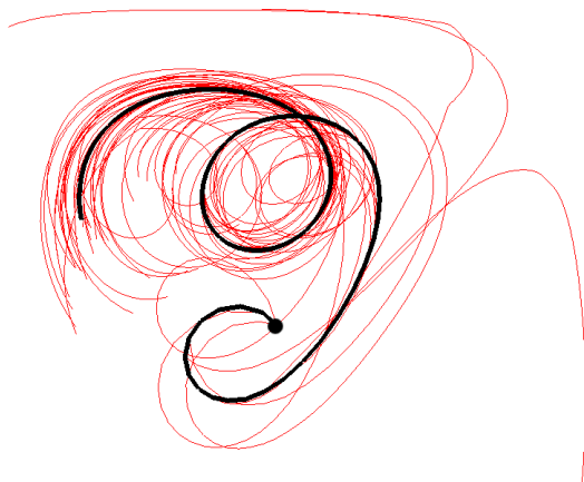
Figure 3: Fluid simulation particle trajectories: Thick black line: full simulation “center-line” trajectory ( v = 0 ; semi-Lagrangian advection). Red thin lines: full simulation basis enrichment trajectories. Bottom 1/4 of the simulation box is not shown. All trajectories correspond to a particle initially located at the center of the simulation box (denoted by the black circle) and integrated using a Runge-Kutta second-order integrator. Same initial external force, followed by control-free motion. 256x256 MAC grid.
