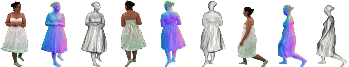
Figure 1: Our system rapidly acquires images under varying illumination in order to compute photometric normals from multiple viewpoints. The normals are then used to reconstruct detailed mesh sequences of dynamic shapes such as human performers.
