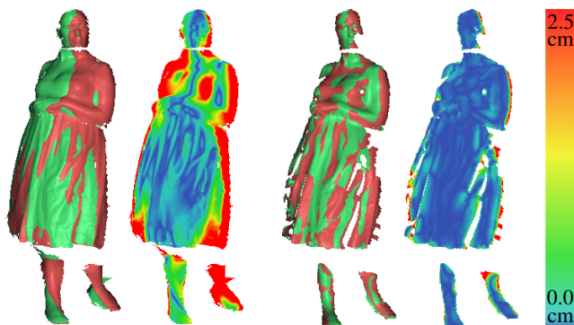
Figure 7: The integrated surfaces before matching (left) are far from each other, while the deformed surfaces after matching (right) are much closer to each other. Within each pair, the leftmost visualization shows the two meshes (in different colors) overlaid on each other, while the rightmost visualization is a color-coding of mesh-to-mesh distance.
