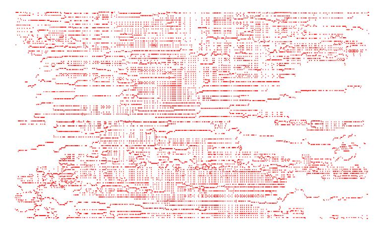
11,849 holes to drill in a programmed logic array Reference: http://www.tsp.gatech.edu
