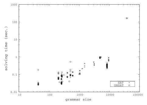
Fig. 8. HAMPI solving time as function of grammar size (number of all elements in all productions), on 1,367 inputs from the Wassermann and Su [Wassermann and Su 2007] dataset. The size of the string variable was 4, the smallest at which HAMPI finds all satisfying assignments for the dataset. Each point represents an input; shapes indicate SAT/UNSAT. Section 5.1 describes the experiment.
