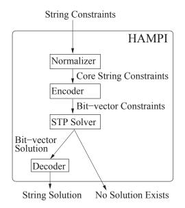
Fig. 3. Schematic view of the HAMPI string constraint solver. Input enters at the top, and output exits at the bottom. Section 3 describes the HAMPI solver.
