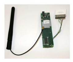
Figure 3: A gumstix-based Nike+iPod surveillance device with wireless Internet capabilities.
