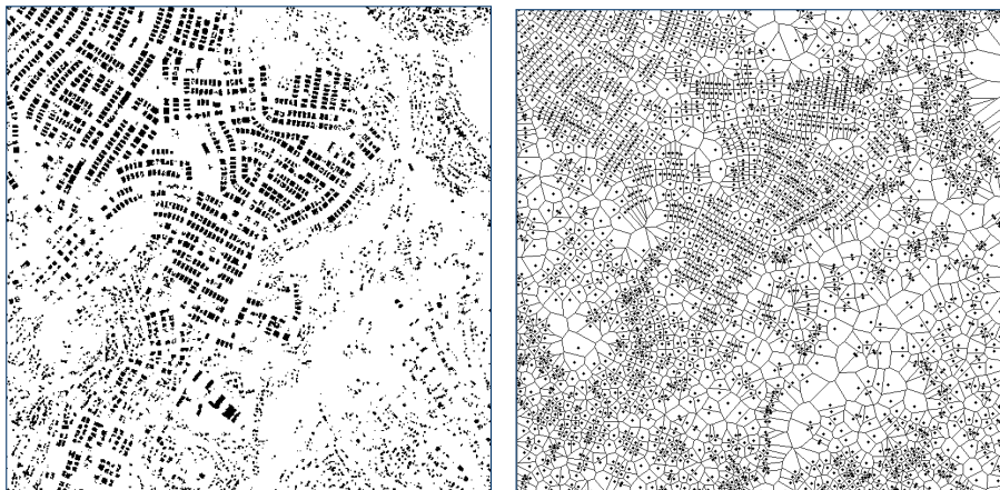
Figure 52: Example for modeling neighboring objects using Voronoi tessellation of a map of buildings detected in an Ikonos image of Ankara.
