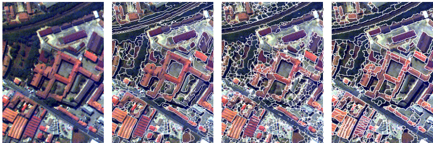
Figure 12: Example segmentation results for the Pavia Centre data set: false color, result of the proposed approach, result of Pesaresi-Benediktsson, result of watershed segmentation.
