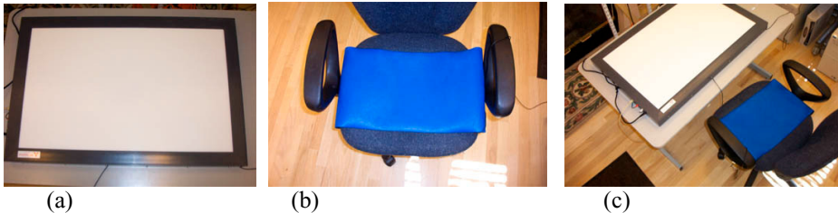
Fig. 1. a) MERL DiamondTouch. b) Conductive mat on chair c) DiamondTouch surface and mat
