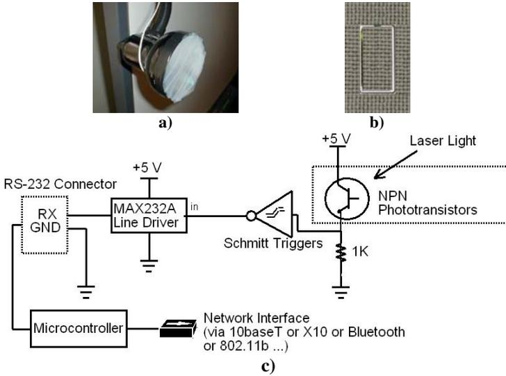
**Fig. 2.** a) A cone-shaped light-sensitive tag. b) A layer of phototransistors replacing a wall plate for a light switch. c) The schematic for the active tag.
