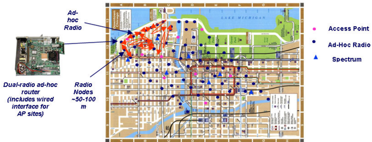
Figure 5.7: Example deployment of an ad-hoc 802.11-based mesh in an urban area.
