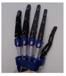
Fig. 1: The 3D-printed 20-DOF anthropomorphic robotic hand.
