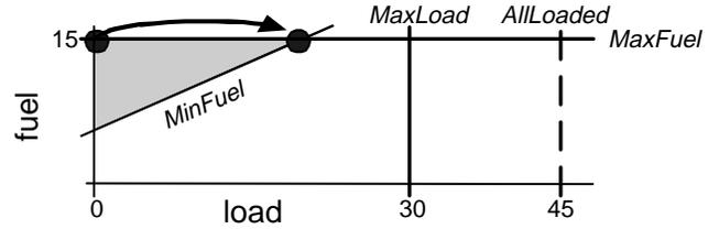
Figure 5: Graphical depiction of the constraints from Figure 2. The shaded area represents solutions to the set of solid-line constraints. The dashed  $\text{AllLoaded}$  constraint causes an inconsistency.
