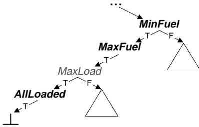
Figure 4: Possible search tree for the constraints from Figure 2. Each node is labeled with the variable set at that node; branchpoints have true (T) and false (F) branches.  $\perp$  indicates an inconsistent constraint set. The bold variables are members of the conflict set.
