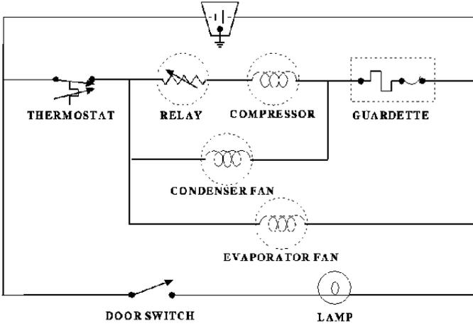
Figure 1: Wiring diagram for a domestic refrigerator
