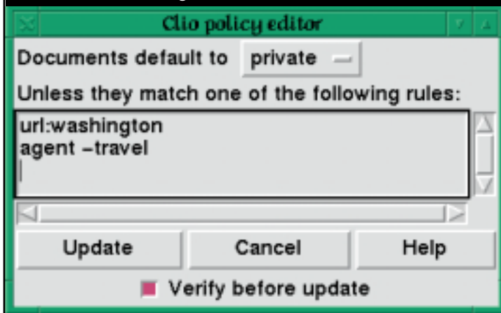
Figure 3. The privacy policy editor interface. Clicking on the Update button puts the policy displayed in the editor window into effect. However, if "verify before update" is enabled, Clío will check for conflicts between the updated policy and existing page privacy settings; if such conflicts are detected, Clío will ask the user to verify that the changes are indeed intended.
