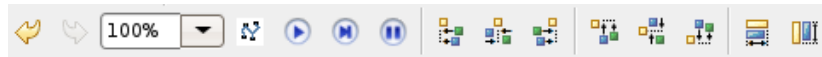
Figure 3.13.: The toolbar of the Inference Visualizer with the actions for undo, redo, the zoom, toggle between automatic and manual layout, the player control, and the alignment.
