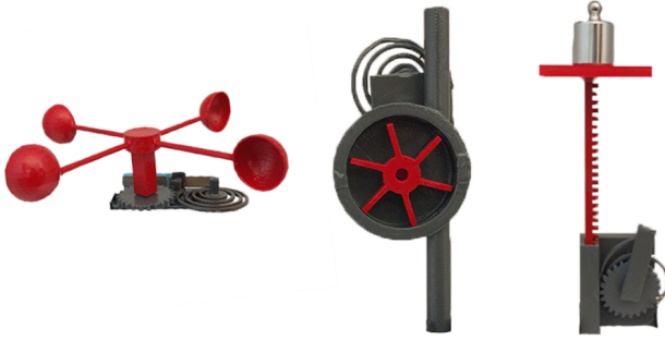
Fig. 2. 3D Printed Wi-Fi Sensors. (a) Anemometer to measure wind speed (b) Flowmeter to measure water speed (c) Scale to measure weight.
