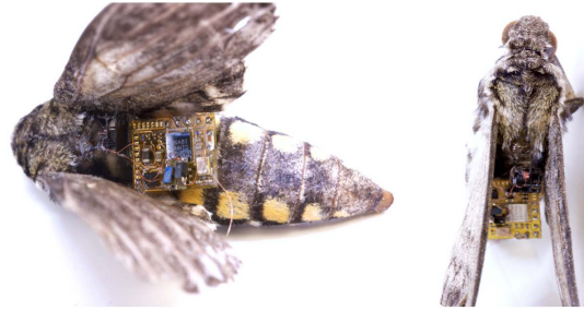
Figure 3: Self-deploying insect-scale sensor attached to the lower thorax of a Manduca sexta moth (see §6).
