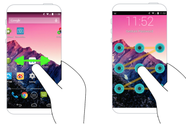
Figure 3: We collect left swipe, right swipe, tap, and long press demonstrations from the Android launcher (left). We collect complex user-defined gestures from the Android lock screen (right).
