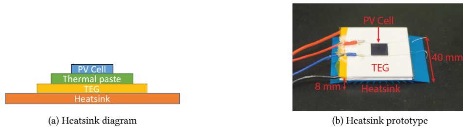
Fig. 8. Heatsink assembly. The PV cell is attached to a thermoelectric generator using thermal adhesive and mounted on an aluminum heatsink allowing the cell to output a stable 1.3 W for 8 hrs.
