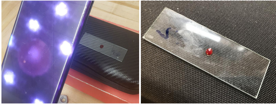
Fig. 1. Generating laser speckle using smartphone LiDAR. (Left) Smartphone LiDAR transmissions as captured by a modified smartphone camera, (Right) close-up of 10 \mu\text{l} of whole blood being tested on a glass slide.
