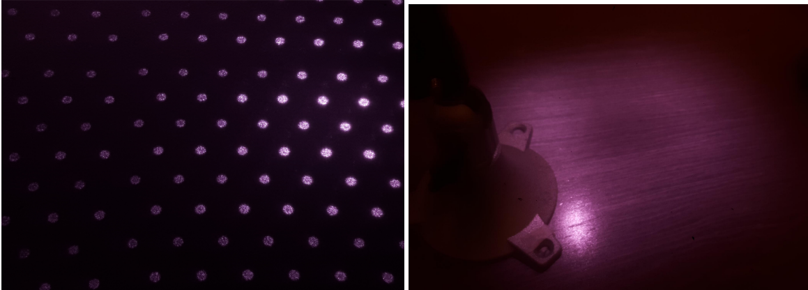
Fig. 3. (Left) Focused LiDAR dot projections from the iPhone 12 and (Right) diffuse laser projection from the Samsung Galaxy Note 10+. The dot projections have a higher power and are more focused allowing for easier speckle pattern extraction.
