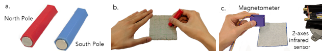
Figure 7: Imaging. (a) 3D printed magnetic pens. (b) Drawing a magnetic image onto a piece of magnetized fabric (c) Decoding the image by scanning a single magnetometer randomly around the image.
