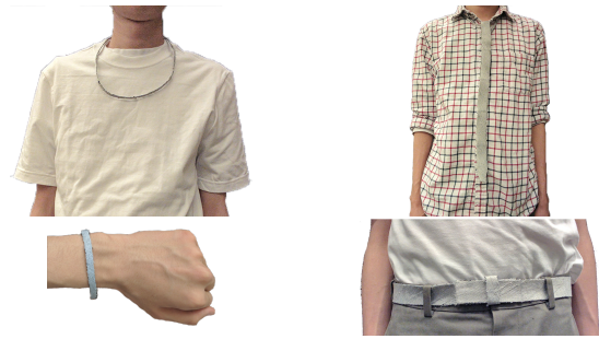
Figure 20: Fashion accessories made with magnetized thread. We create a necklace, necktie, wristband and belt that stores data.
