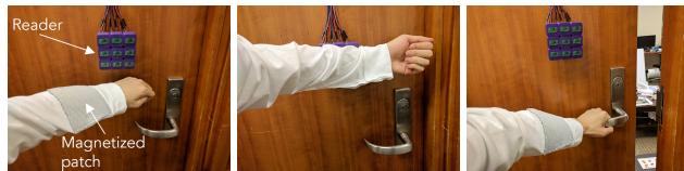
Figure 19: Using a magnetic patch for authentication. Magnetized fabric can be an alternative to RFID cards and used to unlock doors.
