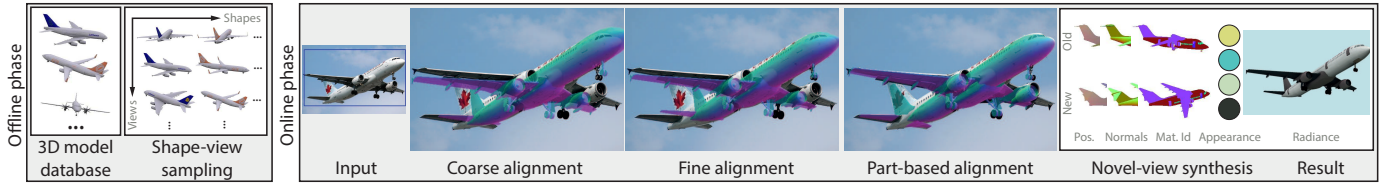
Fig. 6. Overview of our approach comprising an off-line and an on-line phase. The off-line phase samples shapes from a database in many views. In the on-line phase, coarse, fine and per-part 2D-to-3D alignment is performed which is based on a coarse image segmentation derived from user input (scribbles). Finally, novel views are synthesized by rendering the 3D shape in the old and novel views and transferring view-dependent appearance between those images.
