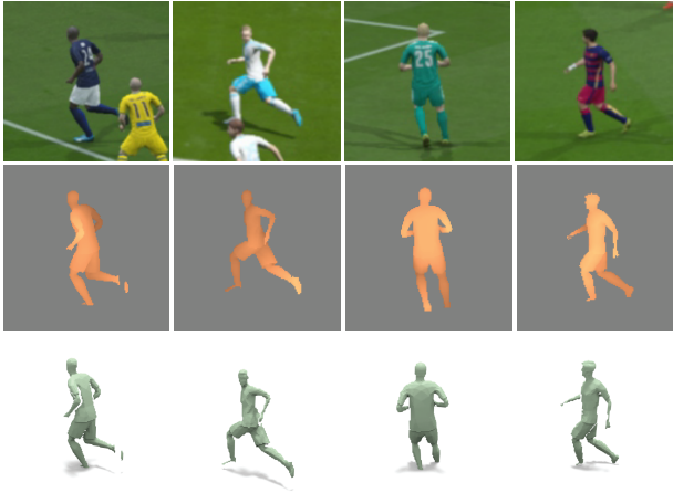
Figure 3. Training data: we extracted images and their corresponding depths while playing a FIFA game. We present several examples here visualized as depth maps and meshes.
