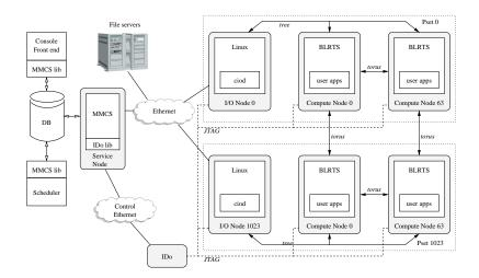
**Fig. 2.** Outline of the Blue Gene/L system software. The computational core is partitioned into 1024 logical processing sets (psets), each with one I/O node running Linux and 64 compute nodes running the custom BLRTS kernel. External entities connect the computational core through two Ethernet networks for I/O and low level management.
