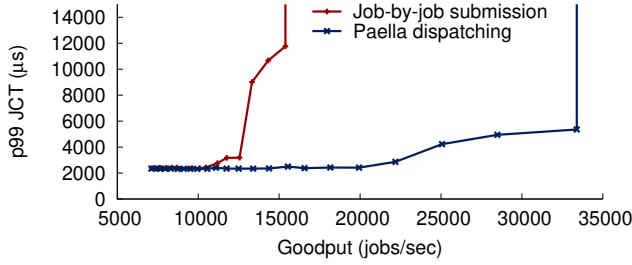
Figure 2. The traditional method of submitting all the kernels of a job together fills all of the GPU’s hardware queues, potentially leaving resources idle while other jobs are queued. In contrast, a well-informed dispatcher (Paella) can increase sustainable throughput while maintaining good tail latency.
