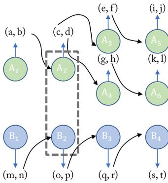
Fig. 8. Vertex-collapsing algorithm to measure time. Each sub-program is a dependency graph and can be represented by a directed graph. Assume two non-adjacent vertices  $A_2$  and  $B_2$  have the same setups, they can be stacked and cut at the same time if there is no cycle after collapsing.
