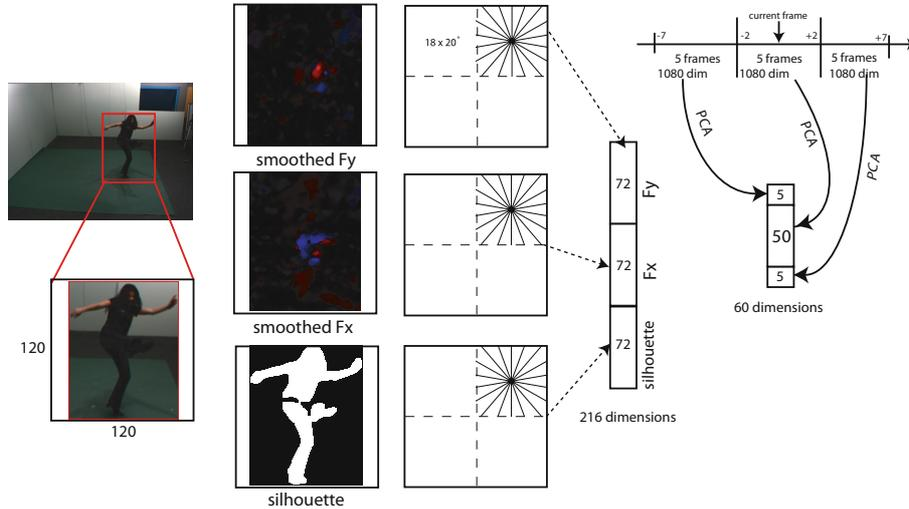
**Fig. 1. Feature Extraction:** Each frame is described by silhouette information, horizontal and vertical optical flow on a normalized size feature extraction window. We histogram all three channels of information by integration over angular slices of subwindows of the bounding box. We then stack information about previous and next frames to model local dynamics of activities.
