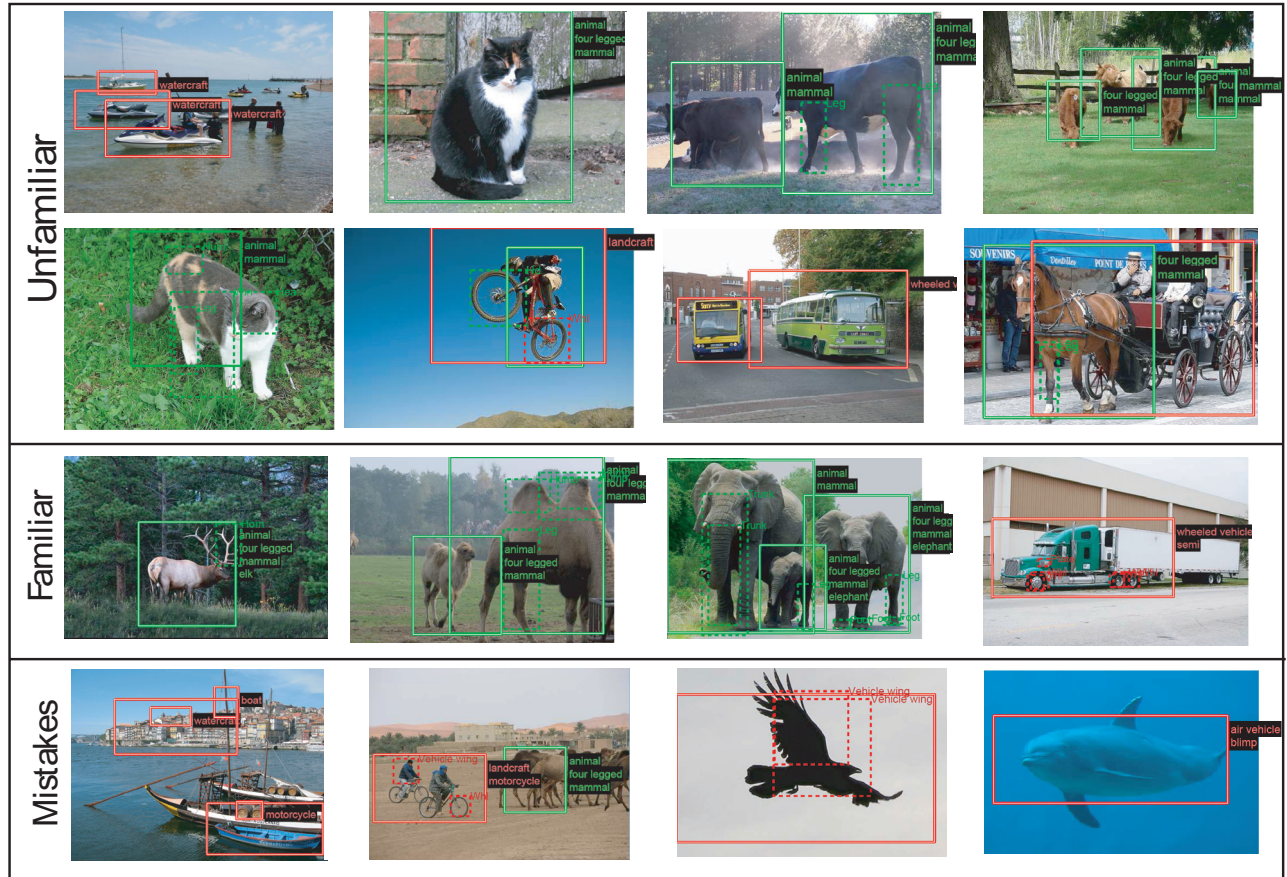
Figure 7. Our system can find animals and vehicles and localize their parts, even if it has never seen them before. The first two rows show examples of detections for animals and vehicles like cows, cats, bicycles, buses, carriages, or horses, that our system never observed. Often times, detected parts help the final detection of unfamiliar objects. For example the the legs of the cows in the first row, or the wheels of the carriage in the second row. Each solid-line bounding box is an object detection above a given threshold ( red=vehicle, green=animal ), and dashed boxes show part detections that helped to find the object (first three letters of part name shown). Black boxes indicate detected categories. The third row depicts examples of detecting familiar objects. The bottom row shows examples of mistakes our system makes. For example predicting vehicle wings for the motorcycle. This is mainly because of the fact that we do not enforce any consistency during localization.
