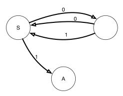
Figure 1: A finite state automaton that accepts strings that have a 1 in some odd location.
