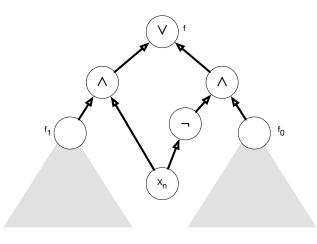
**Figure 1**: Recursive construction of a circuit for *f*.
